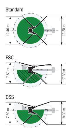
Support width based on center of support leg
