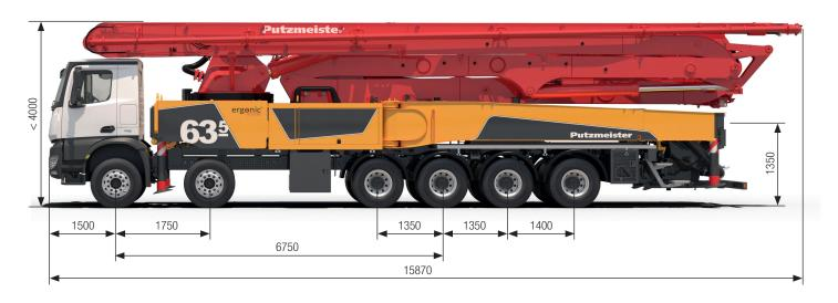
Note: Serial version. Dimensions and weights depend on truck, pump model and equipment.
